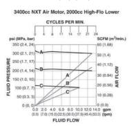
A = 7.0 bar (100 psi) air pressure B = 4.9 bar (70 psi) air pressure
