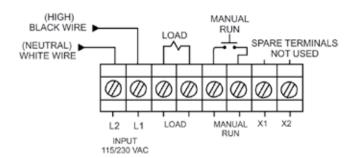
**NOTE:** Two spare terminals x1 and x2 are provided for customer convenience. They are not connected on the board and can be used for any terminations or junctions.
